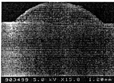
(a) Cladding speed=1.5mm/s, 5mm away from the beginning
